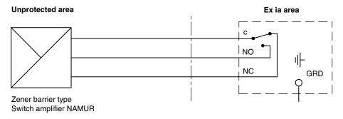
Fig. 6: Operation of pressure switches in intrinsically safe areas
