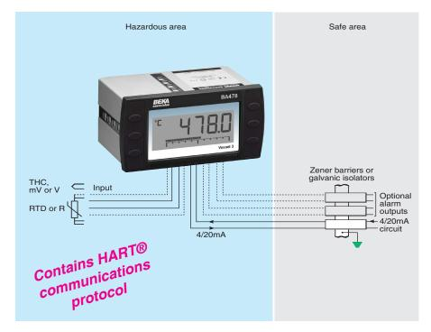
The BA478C is a second generation panel mounting intrinsically safe loop powered indicating temperature transmitter. It provides an accurate local digital temperature display, plus a 4/20mA output that may be scaled to represent any temperature range. The BA478C incorporates HART® digital communication, diagnostics and a robust enclosure with an IP66 front.
