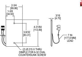
The Series TE-WSS Stainless Steel Wall Plate Temperature Sensor measures the ambient air temperature in classrooms and industrial environments.
