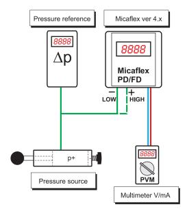
User adjustment in 5 points is possible to perform on MF-FD with software version 4.20 or later for the motherboard (P08) and version 4.10 or later for display module (P09). The software version is shown in parameter P08 and P09. For earlier version, use operating manual Mi-336 which is available on www. micatrone se
