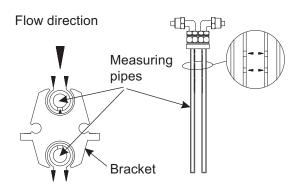
The measuring pipes are holed in accordance with reliable standards. The holes face towards the centre of the bracket.
